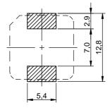
no sensitive traces underneath the component
