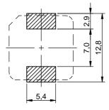
no sensitive traces underneath the component
