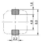
no sensitive traces underneath the component
