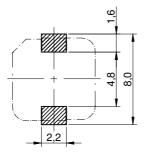
no sensitive traces underneath the component
