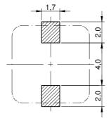
no sensitive traces underneath the component
