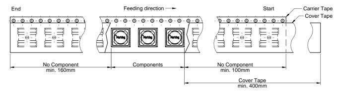
Tolerance packaging is reffered to the international standard IEC 60286-3:2013 Tape width
