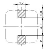
no sensitive traces underneath the component
