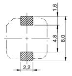
no sensitive traces underneath the component
