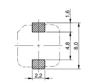
no sensitive traces underneath the component
