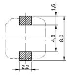
no sensitive traces underneath the component
