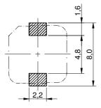
no sensitive traces underneath the component
