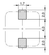
no sensitive traces underneath the component
