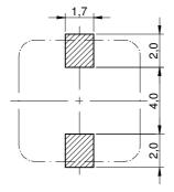
no sensitive traces underneath the component
