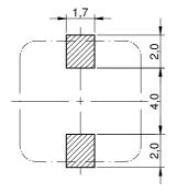
no sensitive traces underneath the component
