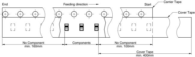
Material Packaging is refered to the international standard IEC 60286-2:2015 Tolerance ± 2,0 min. +1.5
