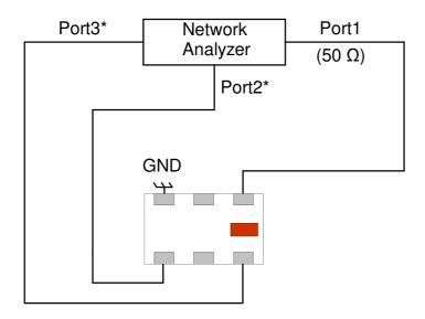
\*Impedance for ports 2 and 3=1/2(Balanced impedance)
