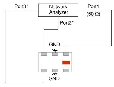
\*Impedance for ports 2 and 3=1/2(Balanced impedance)
