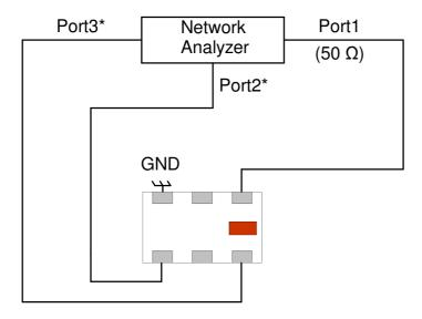
\*Impedance for ports 2 and 3=1/2(Balanced impedance)
