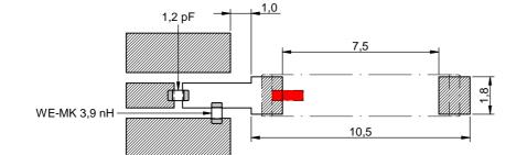
The matching circuit shown has been designed based on the Würth Elektronik evaluation board and cannot be reused. It is recommended to leave a 'Pi' or 'T' type matching circuit space for antenna matching circuit for other boards.
