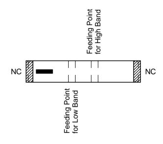
The matching circuit shown has been designed based on the Würth Elektronik evaluation board and cannot be reused. It is recommended to leave a 'Pi' or 'T' type matching circuit space for antenna matching circuit for other boards.
