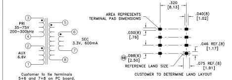
Application of the transformer allows for the leadwires between terminals 5&6 and 7&8 to solder bridge.
