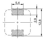
no sensitive traces underneath the component
