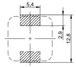
no sensitive traces underneath the component
