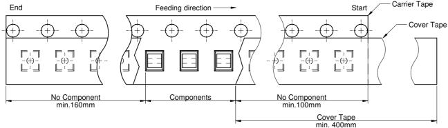
W2 detail B Cover Tape Chip Cavity Sprocket Hole
