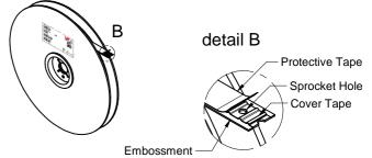
DATE (YYYY-MM-DD) GENERAL TOLERANCE  $\bigcirc$ RoD 006.003 2021-04-23 DIN ISO 2768-1m **WE-VD Disk Varistor** Würth Elektronik eiSos GmbH & Co. KG EMC & Inductive Solutions Max-Eyth-Str. 1 820522511 74638 Waldenburg Germany Tel. +49 (0) 79 42 945 - 0 SIZE/TYPE BUSINESS UNIT www.we-online.com **WÜRTH ELEKTRONIK** 3/7 20 mm eiSos Valid eiSos@we-online.com
