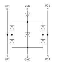
Flow-Thru Design:Route the data lines straight away under the TVS diode I/O pins, that the data signal will not pass through the diode.
