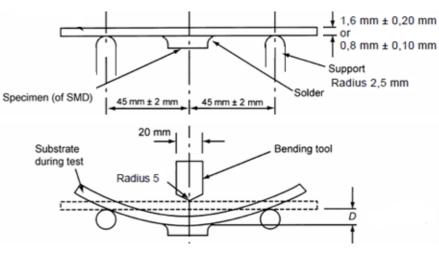
This substrate bending test is for all size of WCAP-CSST.
