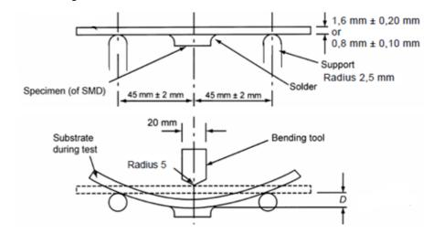
This substrate bending test is for all size of WCAP-CSST.
