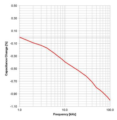
Test Equipment: E4991A or equivalent
