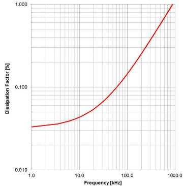
Test Equipment: E4991A or equivalent
