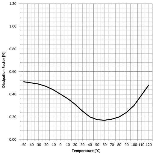
Test Equipment: E4991A or equivalent
