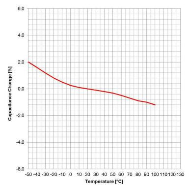
Test Equipment: E4991A or equivalent
