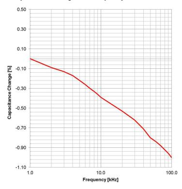
Test Equipment: E4991A or equivalent
