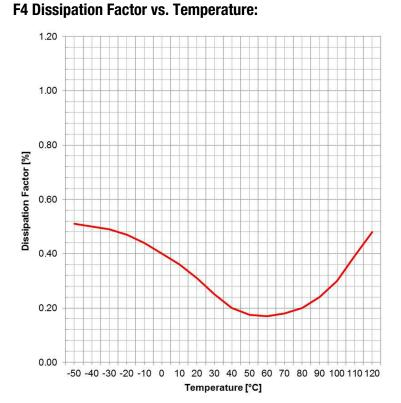
Test Equipment: E4991A or equivalent
