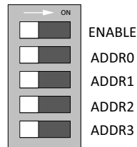
Figure 3-8: Configuration DIP Switch (SW13)
