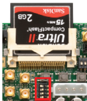
Figure 3: Compact Flash Card Installation and DIP Switch Settings
