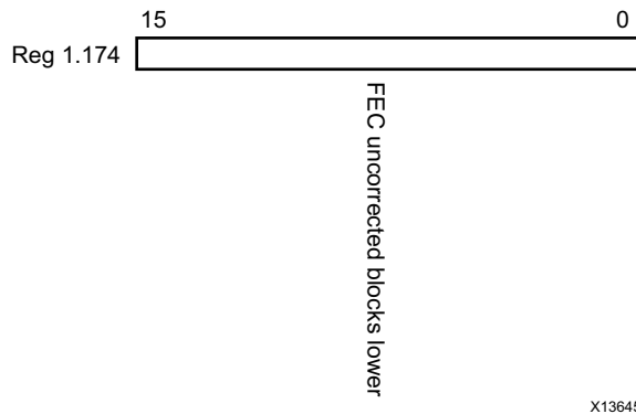
Figure 2-23: 10GBASE-R FEC Uncorrected Blocks (Lower) Register
