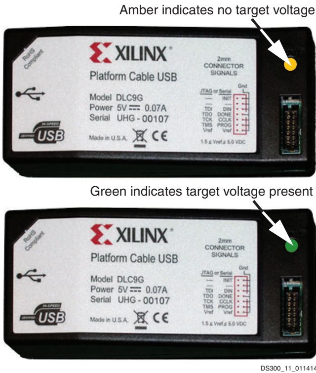
Figure 11: Status LEDs Indicating Target Voltage
