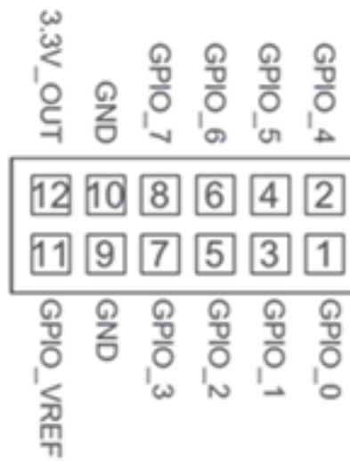
Figure 1-13: GPIO 2x6 Pin Assignments
