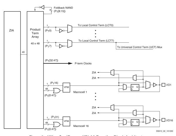
Figure 3: Xilinx CoolRunner XPLA3 Function Block Architecture
