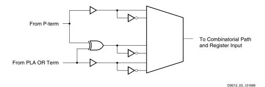
Figure 4: Variable Function Multiplexer
