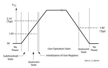
Figure 7: Device Behavior During Power Up
