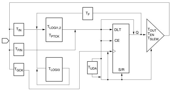
Figure 8: XPLA3 Timing Model
