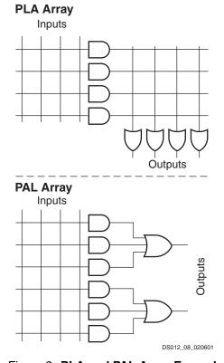
Figure 2: PLA and PAL Array Example
