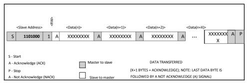
Figure 6-4. Data Read—Slave Transmitter Mode
