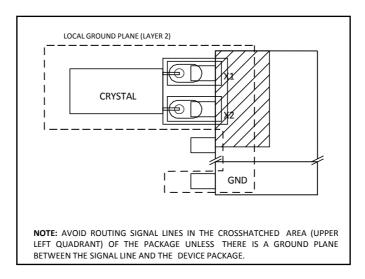
Figure 6-1. Recommended Layout for Crystal
