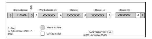
Figure 6-3. Data Write—Slave Receiver Mode
