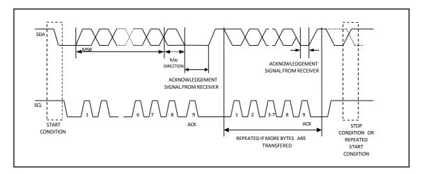
Figure 6-2. Data Transfer on I2C Serial Bus
