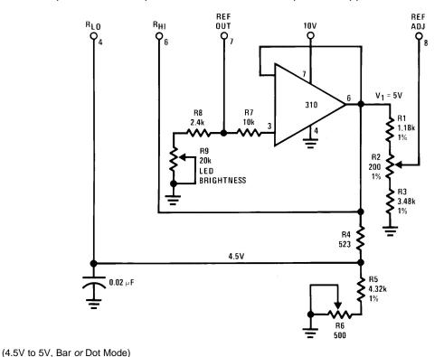
Figure 26. Non-Interacting Adjustments for Expanded Scale Meter
