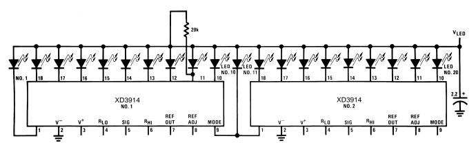
Figure 15. Cascading XD3914 in Dot Mode
