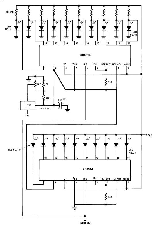
Figure 16. Zero-Center Meter, 20-Segment
