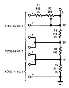
Figure 27. Adjusting Linearity of Several Stacked Dividers
