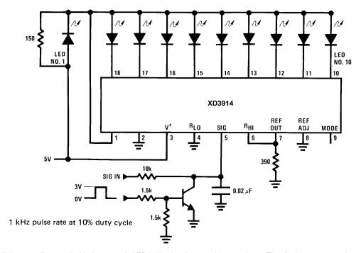
LEDs light up as illustrated with the upper lit LED indicating the actual input voltage. The display appears to increase resolution and provides an analog indication of overrange.
