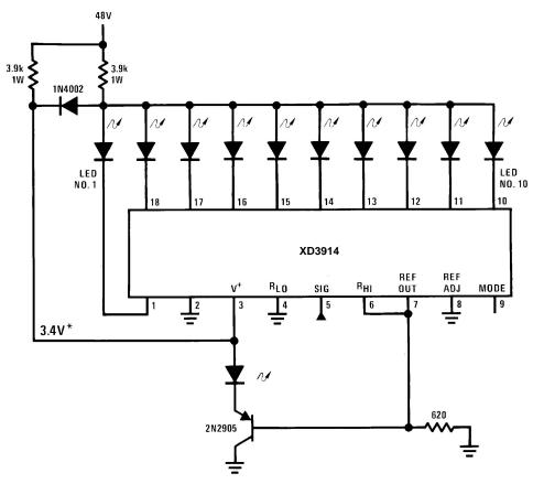
The LED currents are approximately 10mA, and the XD3914 outputs operate in saturation for minimum dissipation. \*This point is partially regulated and decreases in voltage with temperature. Voltage requirements of the XD3914 also decrease with temperature.
