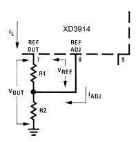
Since the 120µA current (max) from the adjust terminal represents an error term, the reference was designed to minimize changes of this current with V<sup>+</sup> and load changes.
