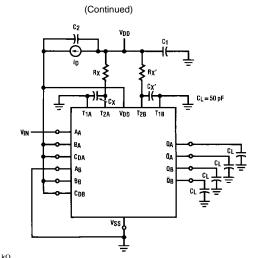
$$\begin{split} R_X &= R_X' = 100 \; k\Omega \\ C_X &= C_X' = 100 \; \mu F \\ C_1 &= C_2 = 0.1 \; \mu F \end{split}$$
