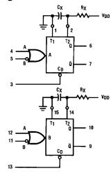
$R_X$  and  $C_X$  are External Components  $V_{DD}$  = Pin 16  $V_{SS}$  = Pin 8
