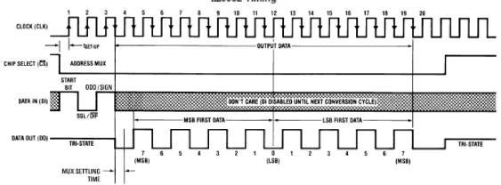
When 2-bit data is set to 1 or 0, only the CHO is converted in single channel.
