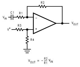
Figure 58. Single-Supply Inverting Amplifier
