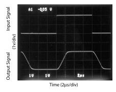
Figure 52. Pulse Response of the XLV324 Circuit in Figure 51
