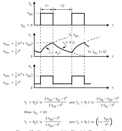
Figure 65. Waveforms of the Circuit in Figure 16
