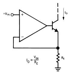
Figure 69. High Compliance Current Sink
