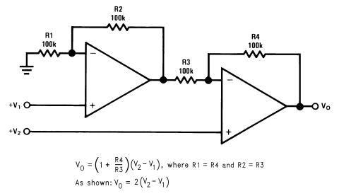
Figure 57. Two-Op-Amp Instrumentation Amplifier
