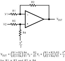
$$\begin{aligned} & V_{OUT} = \left(\frac{R1 + R2}{R3 + R4}\right) \frac{R4}{R1} V_2 - \frac{R2}{R1} V_1 + \left(\frac{R1 + R2}{R3 + R4}\right) \frac{R3}{R1} \cdot \frac{V_1}{2} \\ & \text{for R1} = R3 \text{ and } R2 = R4 \\ & V_{OUT} = \frac{R2}{R1} \left(V_2 - V_1\right) + \frac{V_1^+}{2} \end{aligned}$$
