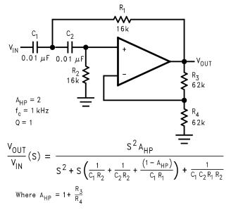
Figure 62. Sallen-Key 2nd-Order Active High-Pass Filter
