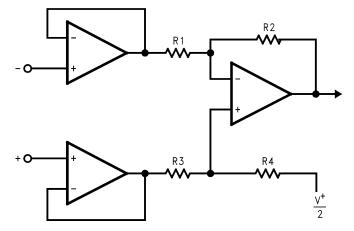
Figure 56. Three-Op-Amp Instrumentation Amplifier
