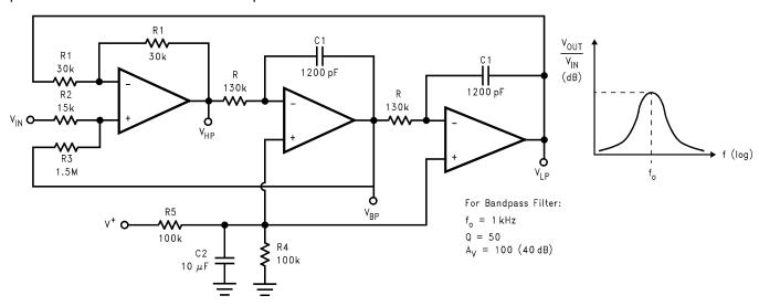
Figure 63. State Variable Active Filter
