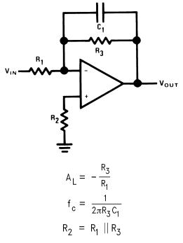
Figure 59. Simple Low-Pass Active Filter
