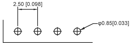
Recommended P.C.B Layout General Tolerance±0.05
