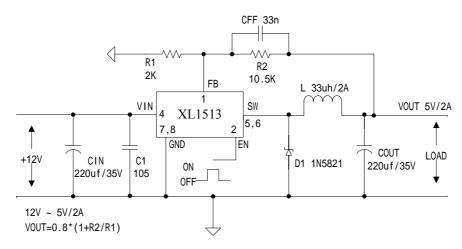
Figure 6. XL1513 System Parameters Test Circuit (12V ~ 5V/2A)
