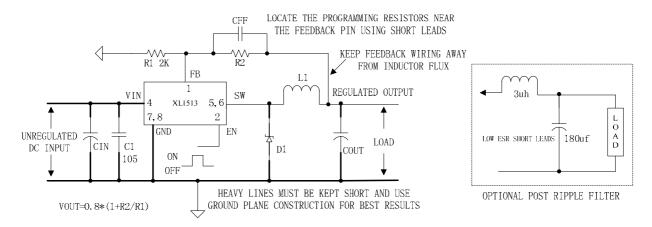
Figure 5. Standard Test Circuits and Layout Guides
