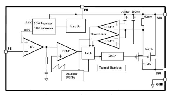
Figure 3. Function Block Diagram of XL1513
