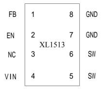
Figure 2. Pin Configuration of XL1513 (Top View)
