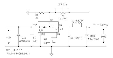
Figure 7. XL1513 System Parameters Test Circuit (12V ~ 3.3V/2A)
