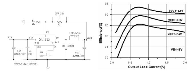
Figure 4. XL1513 Typical Application Circuit
