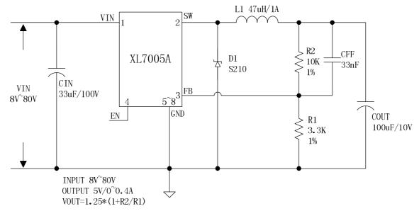
Figure 10. XL7005A System Application (VIN=8V~80V, VOUT=5V/0.4A)
