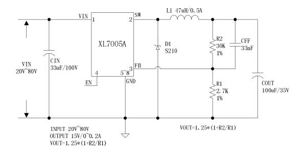
Figure 4. XL7005A Typical Application Circuit
