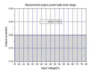
Figure 7. Max output current (VOUT=15V)
