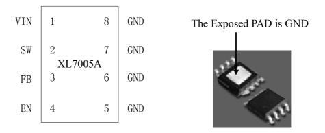
Figure 2. Pin Configuration of XL7005 A(Top View)
