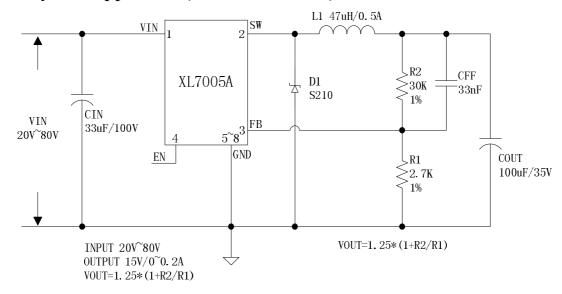
Figure 8. XL7005A System Application (VIN=24V~80V, VOUT=15V/0.2A)
