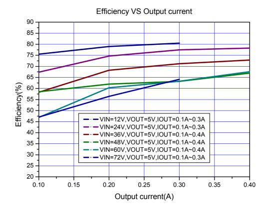
Figure 11. XL7005A System Application (Efficiency VS Output Current)
