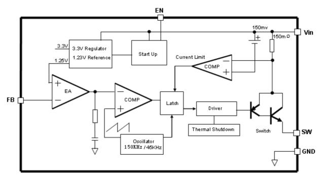
Figure 3. Function Block Diagram of XL7005A
