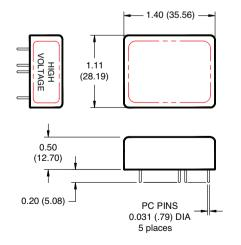
All dimensions are in inches (mm) Tolerance: X.XX ±0.02 (0.51) Pin Tolerance: ±0.005 (0.127) Weight: C01-C20: 1.1oz (31g)
