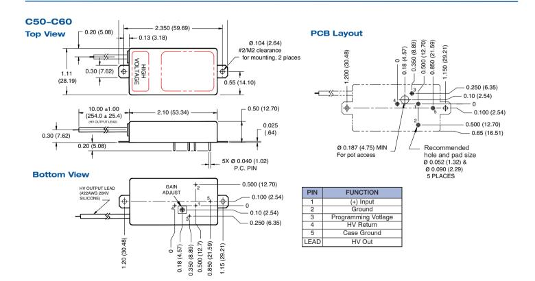
All dimensions are in inches (mm) Tolerance:  $X.XX \pm 0.02$  (0.51) Pin Tolerance:  $\pm 0.005$  (0.127) Weight: C25-C40: 1.3oz (36.8g) C50-C60: 1.8oz (61g)
